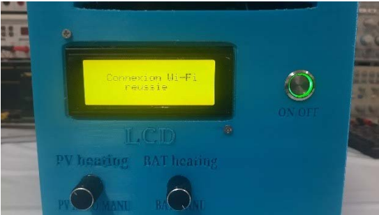
Figure 5. Successful Wi-Fi connection between cooker and local router
